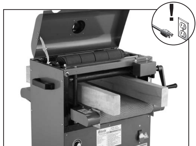
Figure 31. Gauge blocks positioned under pressure rollers and sanding drum.
